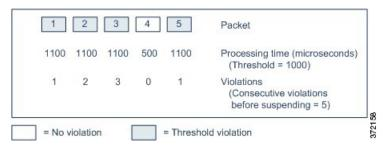
In the above example, the time required to process each of the first three packets violates the rule latency threshold of 1000 microseconds, and the violations counter increments with each violation. Processing of the fourth packet does not violate the threshold, and the violations counter resets to zero. The fifth packet violates the threshold and the violations counter restarts at one.
