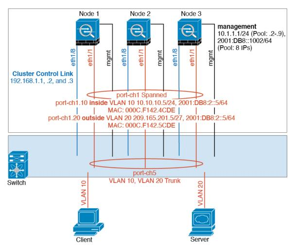
Data traffic from different security domains are associated with different VLANs, for example, VLAN 10 for the inside network and VLAN 20 for the outside network. Each has a single physical port connected to the external switch or router. Trunking is enabled so that all packets on the physical link are 802.1q encapsulated. The is the firewall between VLAN 10 and VLAN 20.
