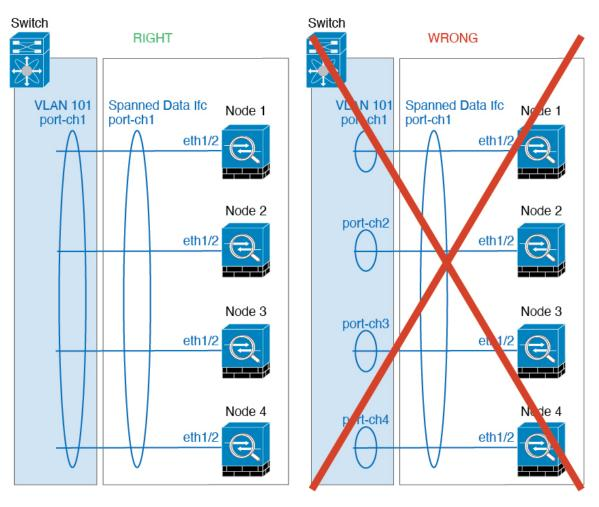
• Device-local EtherChannels—For cluster unit *Device-local* EtherChannels including any EtherChannels configured for the cluster control link, be sure to configure discrete EtherChannels on the switch; do not combine multiple cluster unit EtherChannels into one EtherChannel on the switch.
