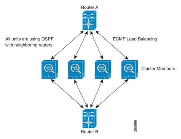
In the above diagram, Router A learns that there are 4 equal-cost paths to Router B, each through a node. ECMP is used to load balance traffic between the 4 paths. Each node picks a different router ID when talking to external routers.
