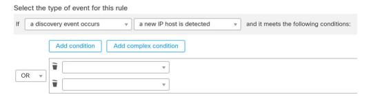
The following graphic shows a correlation rule with one simple condition and one complex condition, joined by the **OR** operator. The complex condition comprises two simple conditions joined by the **AND** operator.
