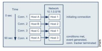
In this example, the system detected a connection that met the basic conditions of the correlation rule, that is, the system detected a connection from a host outside the 10.1.0.0/16 network to a host inside the network. This created a connection tracker.
