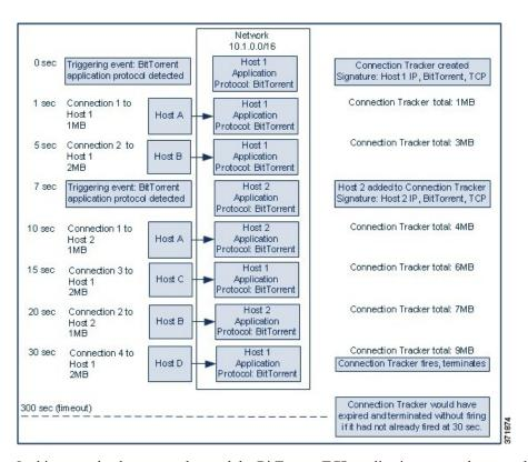
In this example, the system detected the BitTorrent TCP application protocol on two different hosts: Host 1 and Host 2. These two hosts transmitted data via BitTorrent to four other hosts: Host A, Host B, Host C, and Host D.
