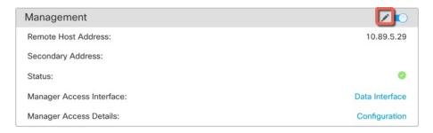
b) In the **Management** dialog box, modify the name or IP address in the **Remote Host Address** field and the optional **Secondary Address** field, and click **Save**.
