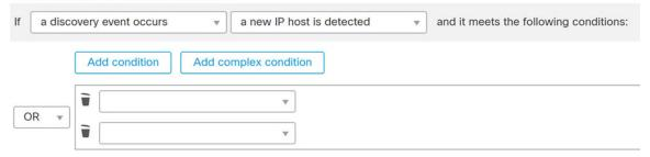
The following graphic shows a correlation rule with one simple condition and one complex condition, joined by the **OR** operator. The complex condition comprises two simple conditions joined by the **AND** operator.
