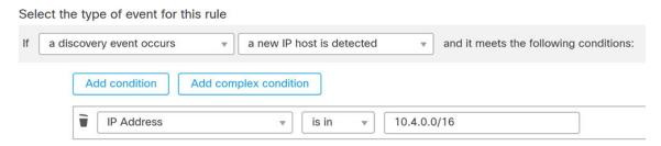
When your construct includes more than one condition, you must link them with an **AND** or an **OR** operator. Conditions on the same level are evaluated together:
