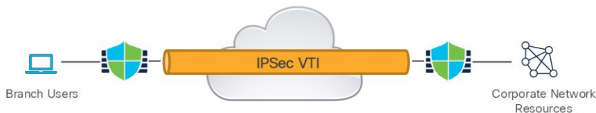
Figure 4. Threat Defense IPsec Virtual Tunnel Interface
