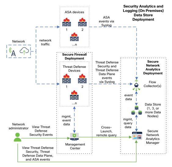
In this deployment, the threat defense and Secure Firewall ASA devices send Firewall events to the Flow Collector. The Flow Collector sends the events to the Data Store for storage. From the management center UI, users can cross-launch to the Manager to view more information about the stored events. They can also query remotely the events from the management center.
