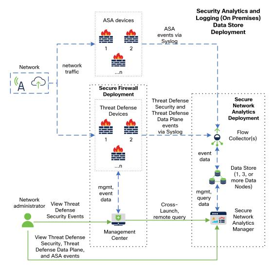
In this deployment, the Firewall Threat Defense and Secure Firewall ASA devices send Firewall events to the Flow Collector. The Flow Collector sends the events to the Data Store for storage. From the Firewall Management Center UI, users can cross-launch to the Manager to view more information about the stored events. They can also query remotely the events from the Firewall Management Center.
