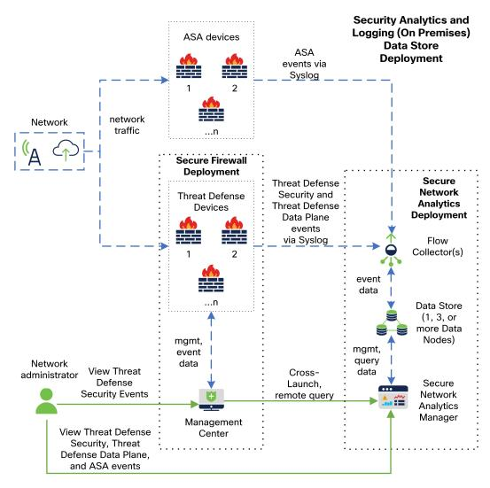
In this deployment, the threat defense and Secure Firewall ASA devices send Firewall events to the Flow Collector. The Flow Collector sends the events to the Data Store for storage. From the management center UI, users can cross-launch to the Manager to view more information about the stored events. They can also query remotely the events from the management center.
