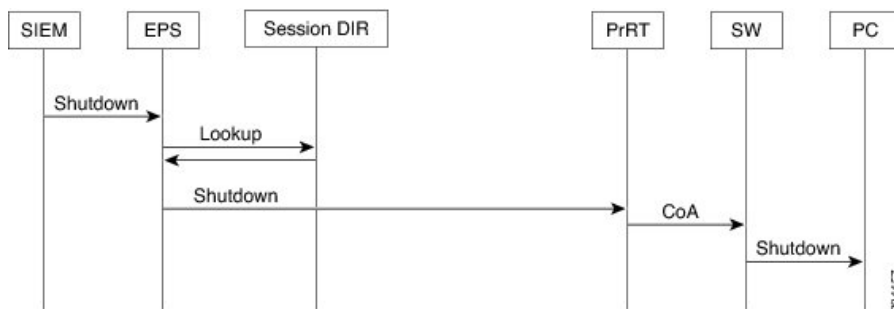
Figure 26: EPS ANC Shutdown Flow
