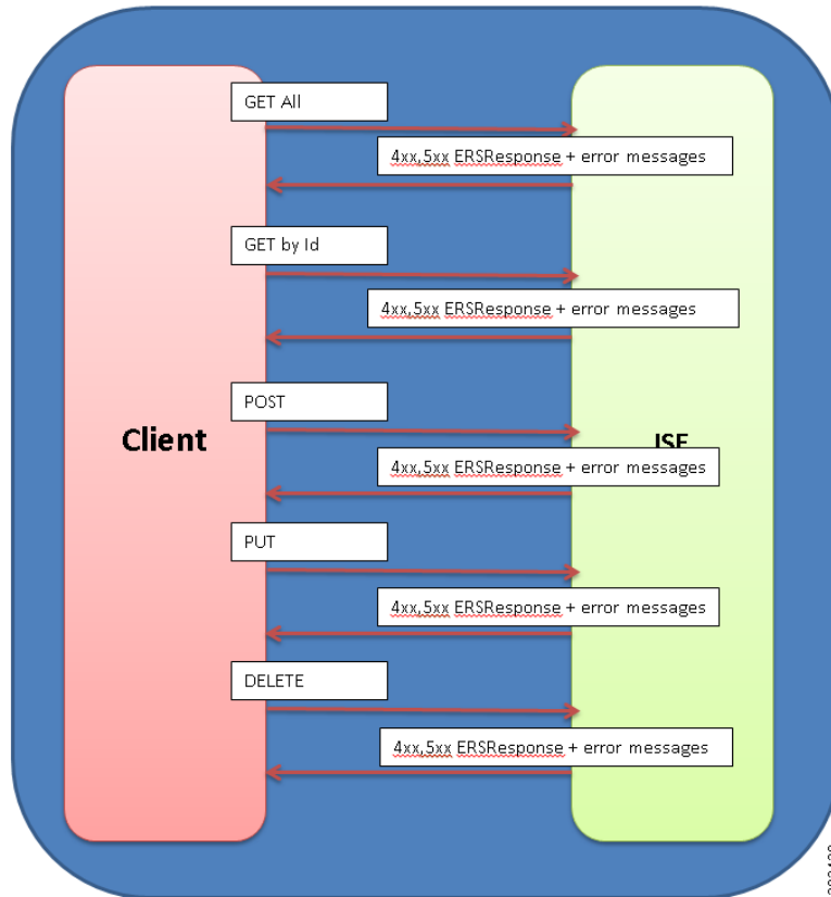
Figure 5-2 ERS Failure Flow Sequence
