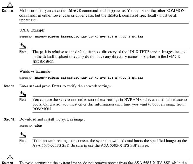
To avoid corrupting the system image, do not remove power from the ASA 5585-X IPS SSP while the system image is being installed.
