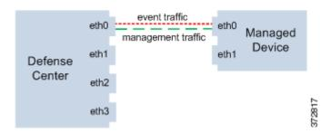
When you use multiple management interfaces, you can improve your performance by dividing the traffic channels over two management interfaces, thus increasing the traffic flow by adding the capacity of both interfaces. One interface carries the management traffic channel and the other carries the event traffic channel. If either interface fails, all traffic reroutes to the active interface and the connection is maintained.
