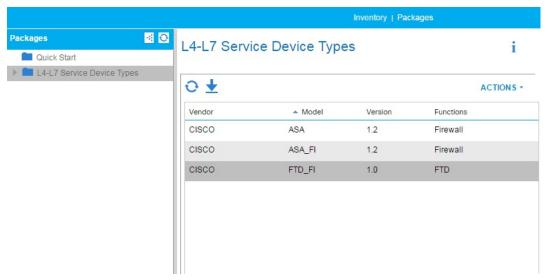
(Optional) In the navigation pane, expand **Device Types** to see the function parameters for the device package.
