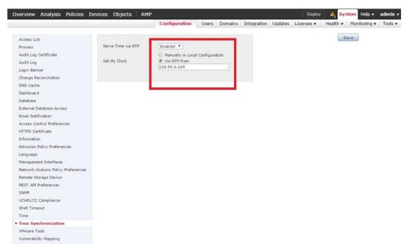
• In the Chassis Manager of the Firepower 41xx and 93xx series appliance, navigate to **Platform** Settings > NTP > Time Synchronization and add the same NTP server:
