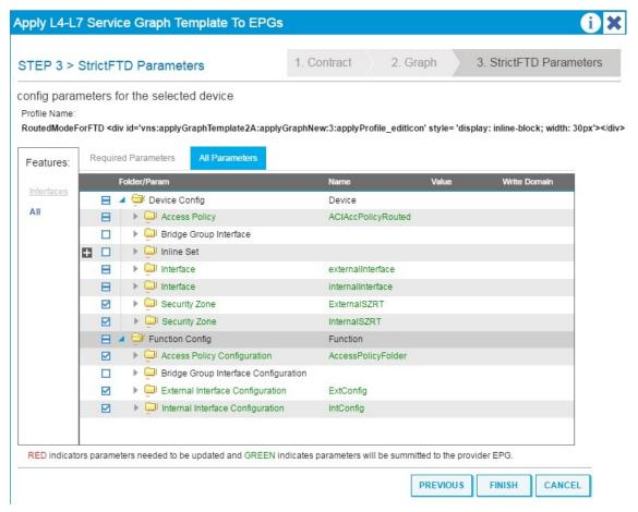
Step 10 Configure the parameters based on your deployment. You can define a function profile based on a built-in template and use that in this step. See the sections on Supported Functions and FTD Deployments, on page 28. Click Finish to attach the contract to the service graph.
