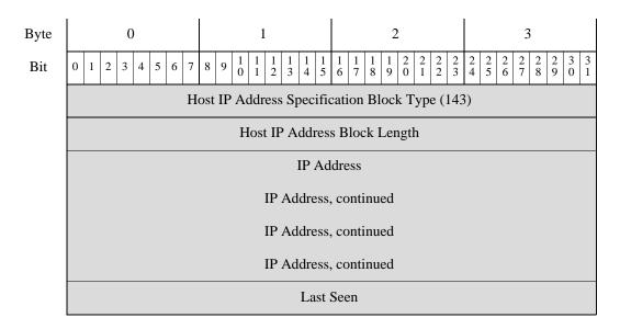
The following table describes the components of the Host IP Address data block.
