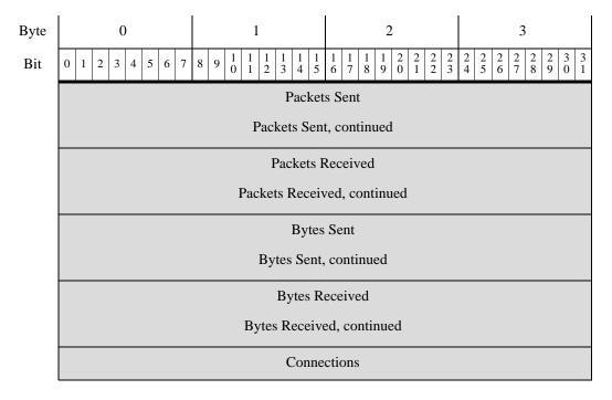
The following table describes the components of the Connection Chunk data block.
