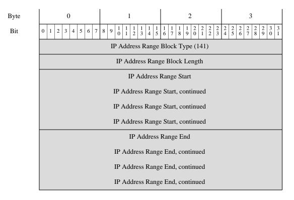
The following table describes the components of the IP Address Range Specification data block.
