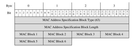
The following table describes the components of the MAC Address Specification data block.
