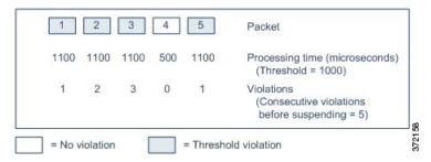
In the above example, the time required to process each of the first three packets violates the rule latency threshold of 1000 microseconds, and the violations counter increments with each violation. Processing of the
