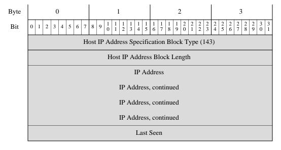
The following table describes the components of the Host IP Address data block.
