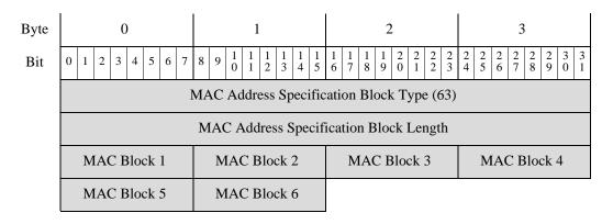
The following table describes the components of the MAC Address Specification data block.
