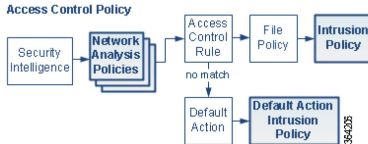
In an inline deployment, the system can block traffic without further inspection at almost any step in the illustrated process. Security Intelligence, the SSL policy, network analysis policies, file policies, and intrusion policies can all either drop or modify traffic.
