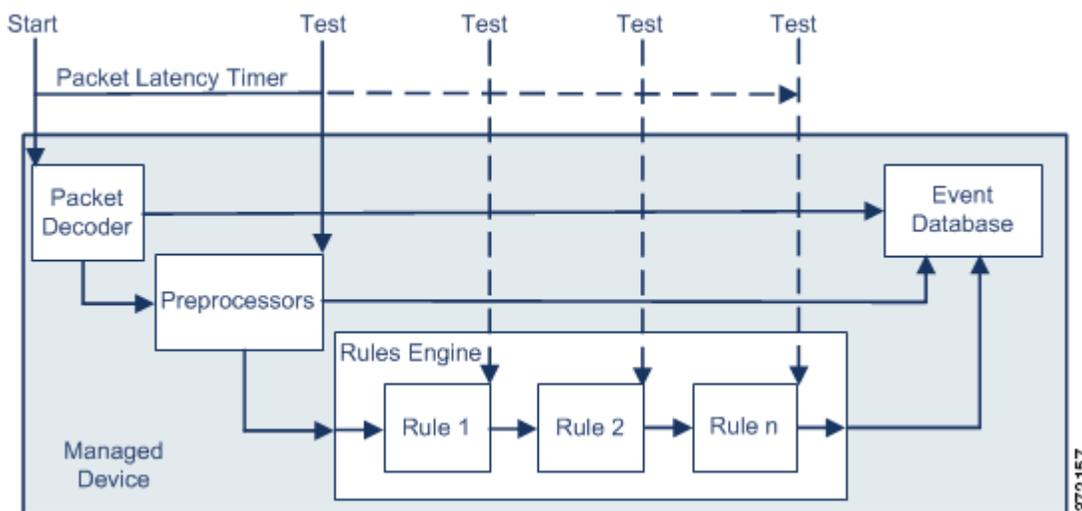
As illustrated in the above figure, packet latency timing is tested at the following test points:
