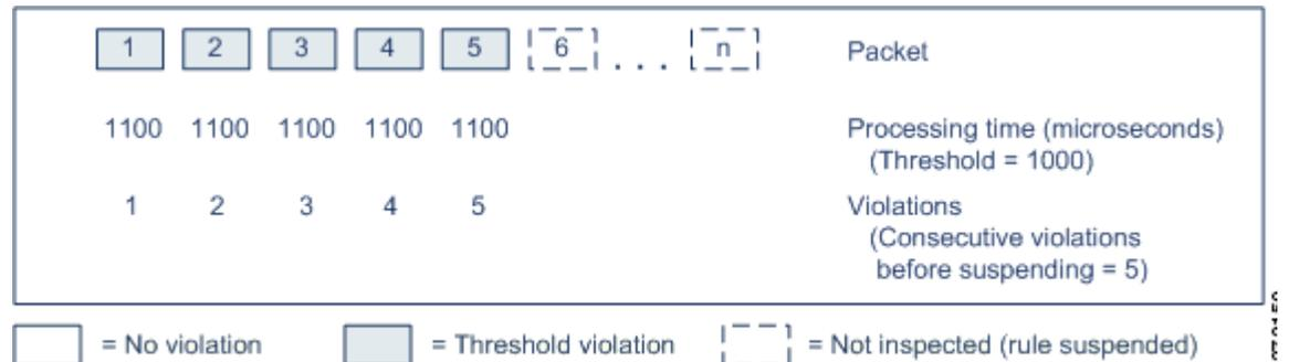
In the second example, the time required to process each of the five packets violates the rule latency threshold of 1000 microseconds. The group of rules is suspended because the rule processing time of 1100 microseconds for each packet violates the threshold of 1000 microseconds for the specified five
