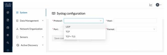
If you select TCP + TLS connection an additional **Set certificate** button is displayed to import a p12 file. This file is to be provided by the administrator of your SIEM solution to secure communications between the Center and the syslog collector.
