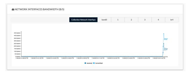
The line charts represent the Collection and the Industrial network interfaces bandwidth with the number of bytes received and sent by the Center per second.
