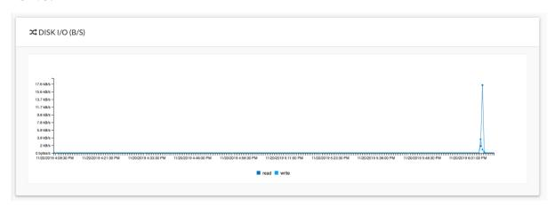
The line chart represents the sensor hard disk usage with the number of bytes read and written per second.
