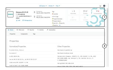
A technical sheet is composed of a top bar and of a list of tabs. The higher part (1) recaps the information found in the right side panel. The rectangular buttons on the right redirect to the corresponding information inside the technical sheet. In a device or a component's technical sheet, you can also edit the element's name, add/remove it to/from a group and add custom properties.
