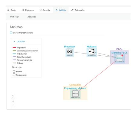
The option "Show inner components" enables an exploded view of the devices.
