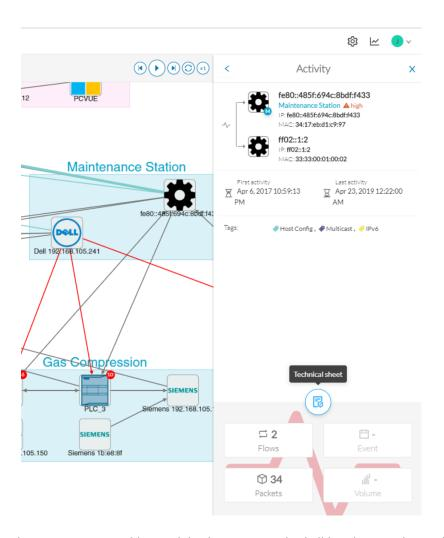
Devices or components with no activity does not mean that it did not have any interaction. In fact, a component can only be detected if at some point it has been involved in a network activity (communication emission/reception). Lack of activity can mean that the other linked component is not part of the preset selected and so doesn't display.
