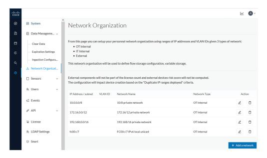
In Cisco Cyber Vision all IP addresses in private format are classified as OT internal by default. Declaring a subnetwork as OT internal is useful in case IP addresses in public format are used in a private network of an industrial site. Conversely, declaring a set of IP addresses as external because they are public will exclude their flows from the database, and exclude their devices from the license device count and the risk score.
