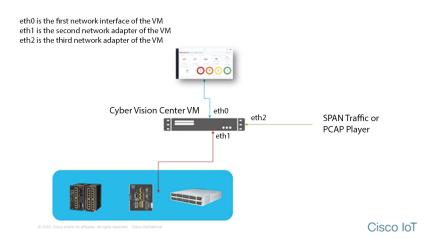
However, in case of incompatibility with the industrial network infrastructure or for limited environments, you can use a single network interface (eth0).
