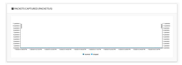
This line chart represents the number of packets that the sensor captures on the Industrial network interface (in bytes per second). It also shows dropped packets, but the value should be zero. If the dropped line shows activity, the sensor is overloaded and is not capturing traffic.
