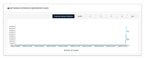
The line charts represent the Collection and Industrial network interfaces bandwidth with the number of bytes received and sent by the Center per second.
