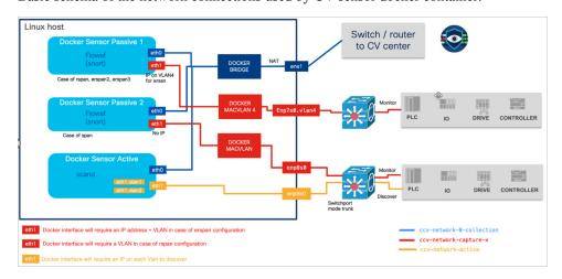
This is an example of a host with two passive Docker sensors (to monitor two different sources of traffic) and one active Docker sensor that can discover two VLANs.
