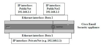
Using Virtual Gateway addresses, a configuration like the one shown in the following figure is also possible.
