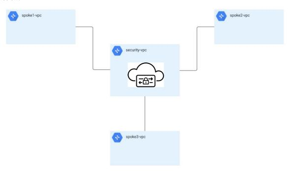
Multicloud Defense orchestrates the creation of the Service VPC and the peering with the Spoke VPCs. Multicloud Defense also provides the ability to update the routing tables in Spoke VPCs to route traffic to
