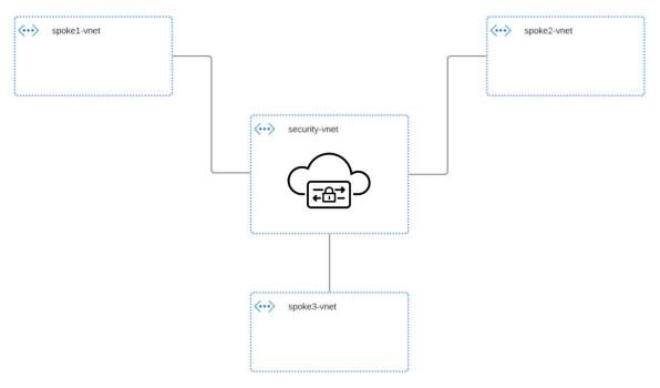
Multicloud Defense orchestrates the creation of the Service VNet and does VNet peering with the Spoke VNets. Multicloud Defense also provides the ability to update the routing in Spoke VNets to route traffic to
