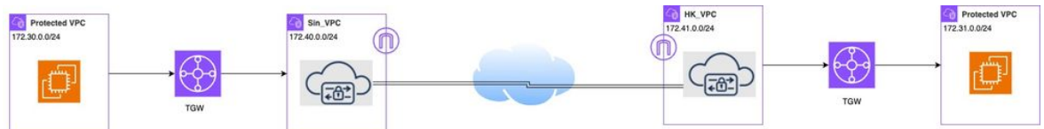
Figure 1: Topology of VPN Site-to-Site Communication
