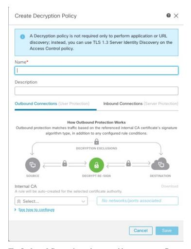
The **Outbound Connections** tab page enables you to create **Decrypt - Resign** rules. These rules require an internal certificate that you can either create beforehand (using **Objects > Object Management > PKI > Internal CAs**) or you can create them as part of the outbound connection rule.
