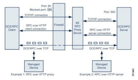
The Microsoft IIS proxy server and the DCE/RPC server can be on the same host or on different hosts. Separate proxy and server options provide for both cases. Note the following in the figure:
