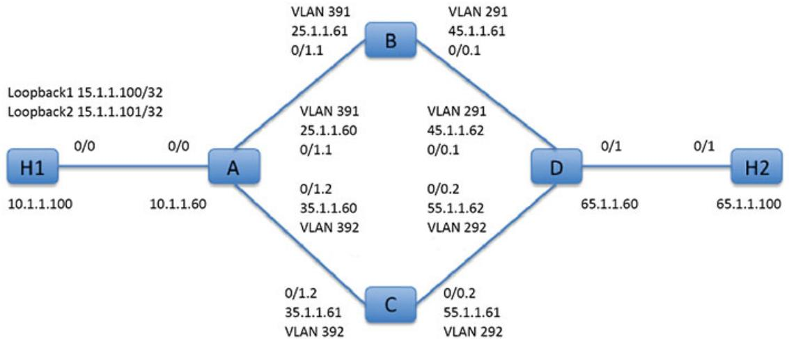
First, we will start with the basic configuration for all the devices involved in the set-up. Here, A, B, C, and D represent ASA devices, and H1 and H2 represent IOS routers.
