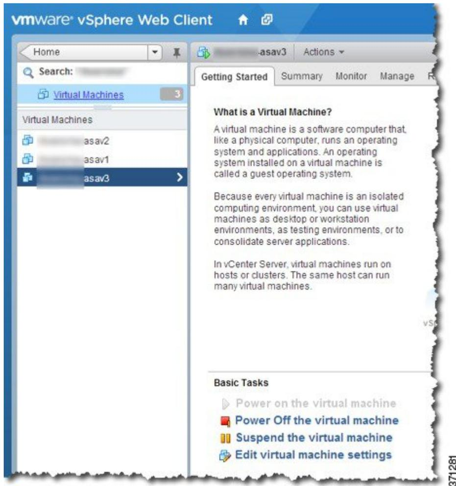
**Step 10** If the ASAv machine is not yet running, click **Power On the virtual machine**.
