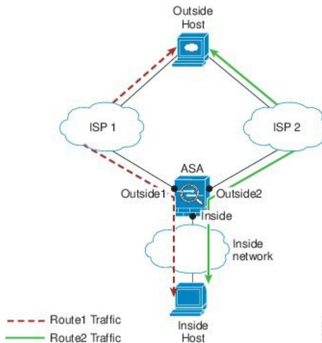
**Non-Zoned Problem:** Load-balancing across interfaces is not possible; you can only load-balance with equal cost routes on one interface.
