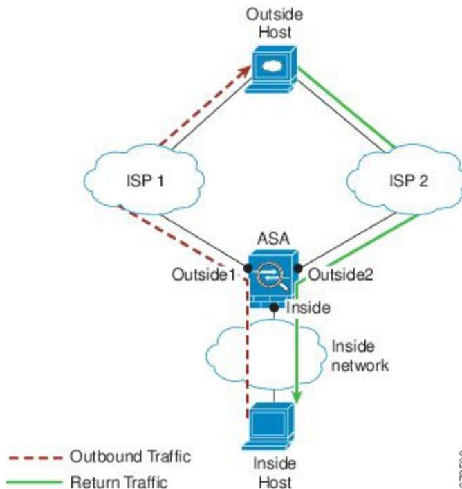
**Non-Zoned Problem:** The ASA maintains the connection tables on a per-interface basis. When the returning traffic arrives at Outside2, it will not match the connection table and will be dropped. For an ASA cluster, asymmetric routing when the cluster has multiple adjacencies to the same router can lead to unacceptable traffic loss.
