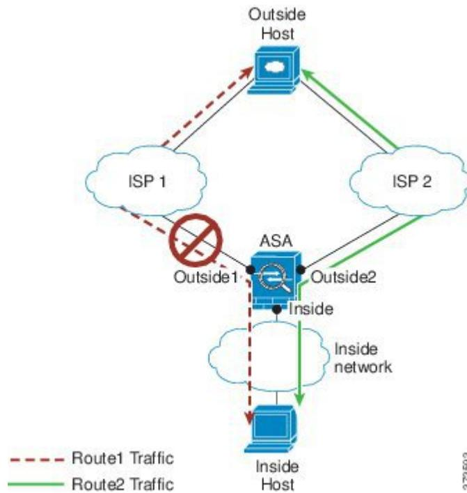
**Non-Zoned Problem:** The connection between the inside and outside host will be deleted; a new connection must be established using a new next-best route. For UDP, the new route will be used after a single packet drop, but for TCP, a new connection has to be reestablished.
