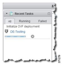
When it is finished, you see the Deploy OVF Template completion status.
