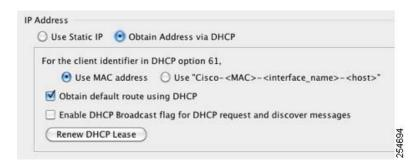
a. To force a MAC address to be stored inside a DHCP request packet for option 61, click the Use MAC Address radio button.
