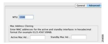
Step 4 To set the MTU or to enable jumbo frame support (supported models only), enter the value in the MTU field, between 300 and 9198 bytes (9000 for the ASAv).
