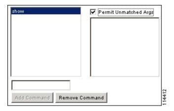
• For commands that are a single word, you *must* permit unmatched arguments, even if there are no arguments for the command, for example **enable** or **help** (see the following figure).
