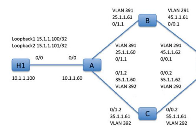
First, we will start with the basic configuration for all the devices involved in the set-up. Here, A, B, C, and D represent ASA devices, and H1 and H2 represent IOS routers.
