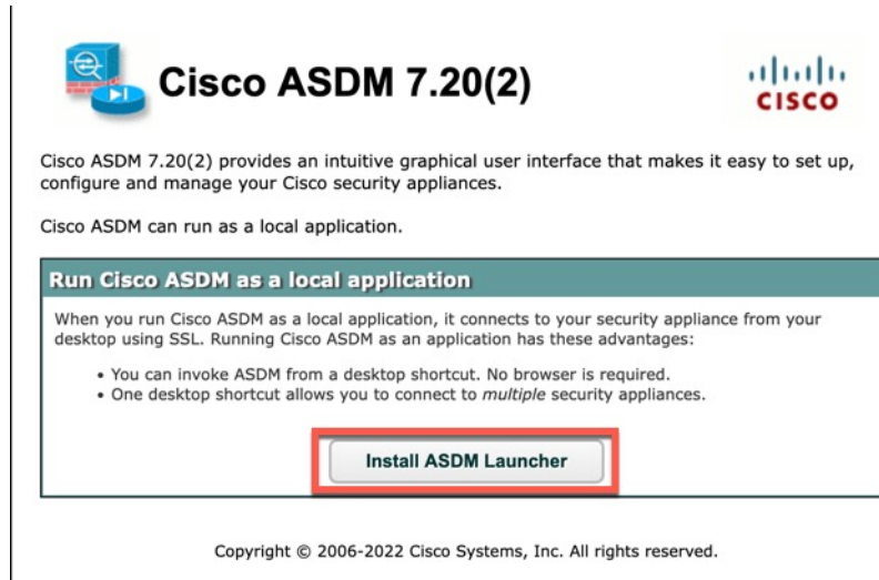
Figure 1: Install ASDM Launcher
