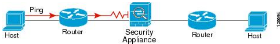
Figure 5: Ping Failure Because the ASA is Not Translating Addresses
