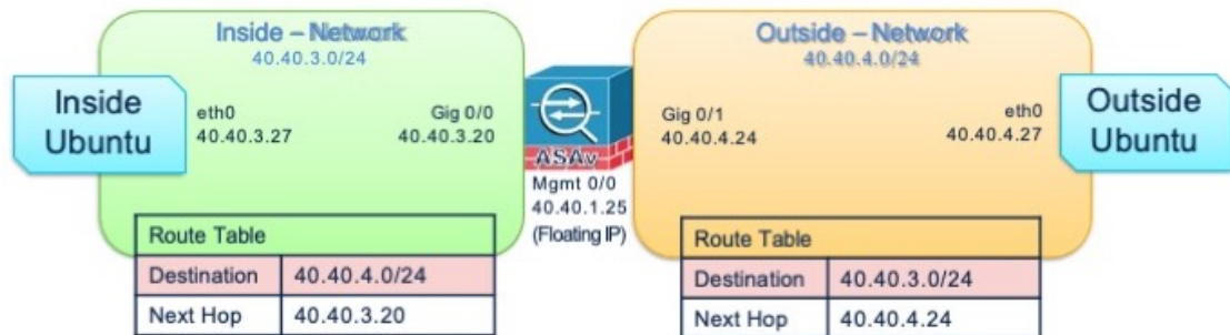
Figure 2: Sample ASAv on OpenStack Deployment
