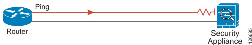
Figure 82-2 Ping Failure at the ASA Interface
