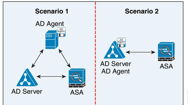
As shown in [Figure 36-3](#), you can deploy the Identity Firewall components to support redundancy. Scenario 1 shows a deployment with multiple Active Directory servers and a single AD Agent installed on a separate Windows server. Scenario 2 shows a deployment with multiple Active Directory servers and multiple AD Agents installed on separate Windows servers.
