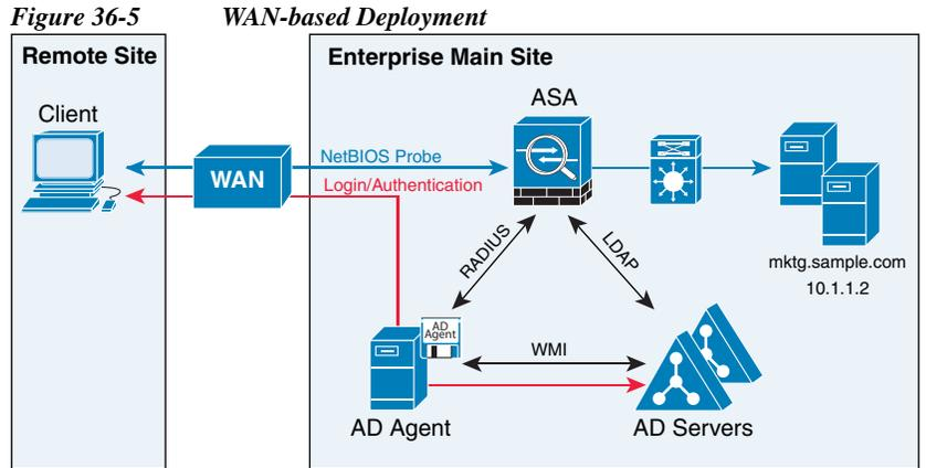
Figure 36-6 also shows a WAN-based deployment to support a remote site. The Active Directory server is installed on the main site LAN. However, the AD Agent is installed and accessed by the clients at the remote site. The remote clients connect to the Active Directory servers at the main site over a WAN.
