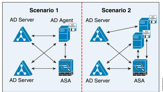
As shown in [Figure 36-4](#), all Identity Firewall components—Active Directory server, the AD Agent, and the clients—are installed and communicate on the LAN.
