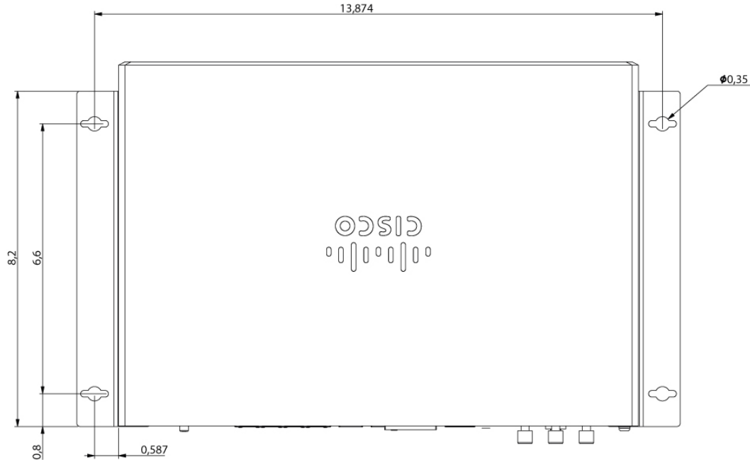
Figure 31: Mounting hole pattern for C8235-G2
