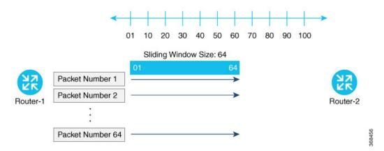
Packets with sequence numbers that fall to the left of the sliding window range are considered old or duplicates, and the destination drops them. The destination tracks the highest sequence number it has received, and adjusts the sliding window when it receives a packet with a higher value.
