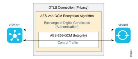
The following are the control plane security components, which function in the privacy provided by DTLS or TLS connections:
