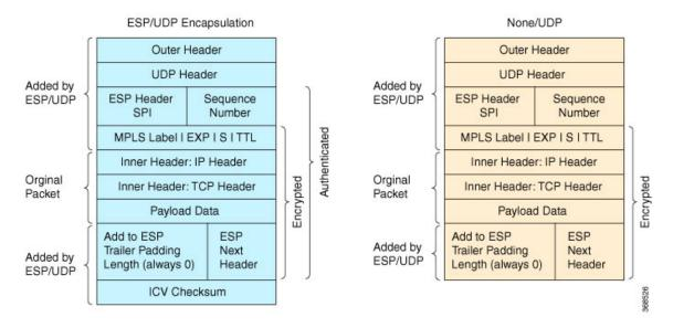
Note that Cisco SD-WAN devices exchange not only the encryption key (which is symmetric), but also the authentication key that is used to generate the HMAC-SHA1 digest. Both are distributed as part of the TLOC properties for a router.
