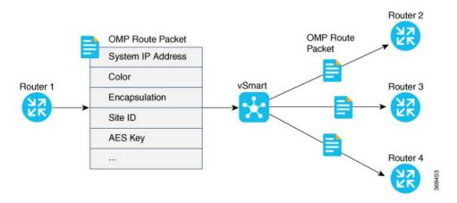
If control policies configured on a vSmart controller limit the communications channels between network devices, the reachability advertisements sent by the vSmart controller contain information only for the routers that they are allowed to exchange data with. So, a router learns the keys only for those routers that they are allowed to communicate with.
