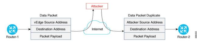
As a counter to such attacks, the Cisco SD-WAN overlay network software implements the IPsec anti-replay protocol. This protocol consists of two components, both of which protect the integrity of a data traffic stream. The first component is to associate sequence numbers with each data packets. The sender inserts a sequence number into each IPsec packet, and the destination checks the sequence number, accepting only packets with
