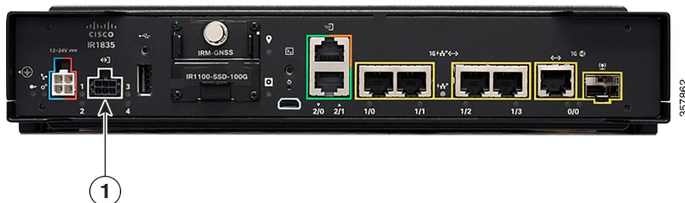
Digital IO is similar to the alarm in and alarm out features supported on Cisco Industrial Ethernet (IE) Series switches and Cisco Industrial Router (IR) Series routers. The differences are that the alarm in is a dedicated input and the alarm out is a dedicated output, whereas the digital IO ports can be used for input or output. alarm out includes a relay to provide normally open (NO) or normally closed (NC) terminals.
